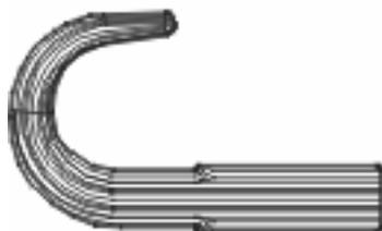
A forged hook has the grains in line similar to the machined hook, but the grains follow the shape of the hook. Rather than acting as “crack here” lines, the lines in the forged hook make the material more malleable and can be described as “bend along here” lines. In an overload situation, the hook will bend without breaking.
