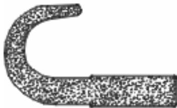
When an object is cast, the metal flows into a mould in no particular order, so the grains tend to be somewhat disjointed. This can make the material brittle. Though it is strong enough for normal applications, in an overload situation, the end of the hook is likely to break off.
